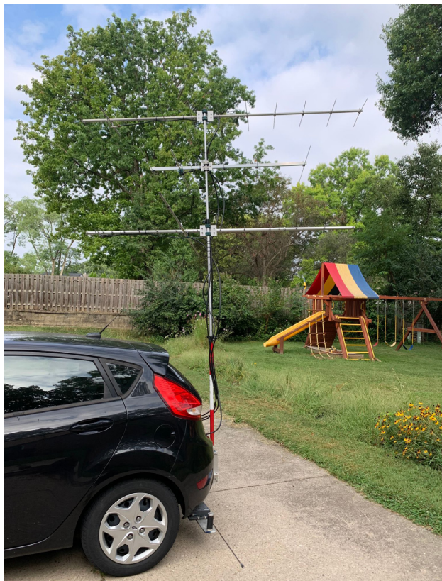
Figure: Rover mast installed with four bands (6-432) at full height.
