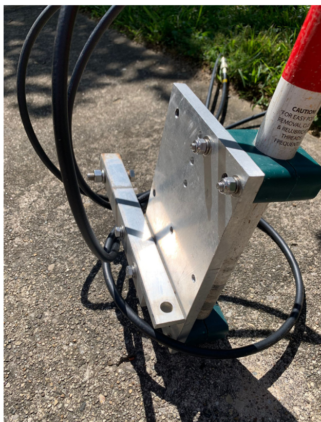
Figure: Hitch receiver mount for mast made from telescoping surveying pole.
