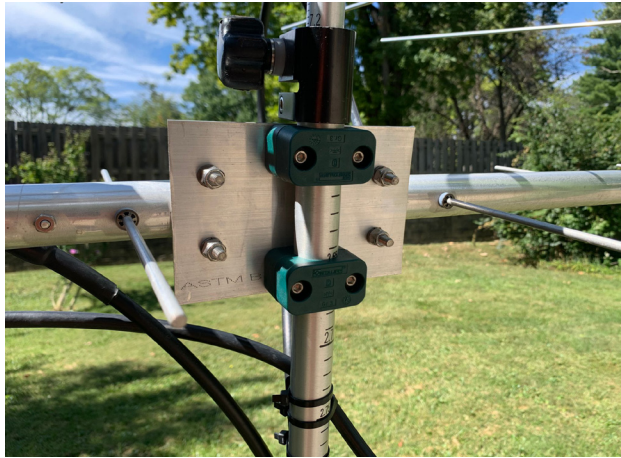
Figure: Boom-to-mast bracket with Stauff mast clamps.
