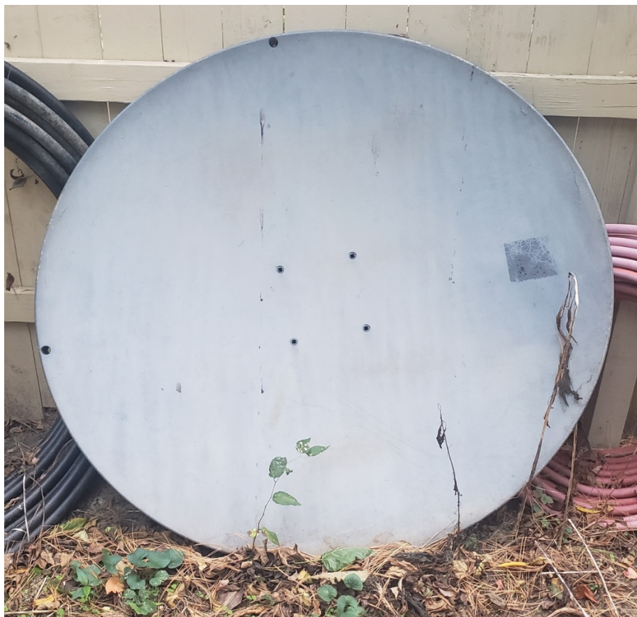
Dish used for this project is a 4-foot diameter offset feed
