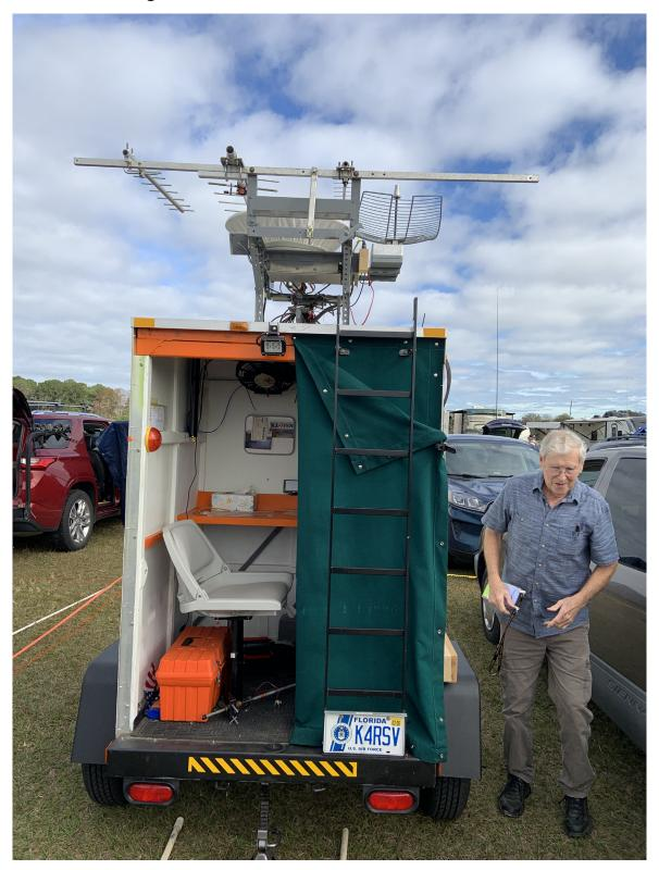
The fan inside the trailer in the upper left corner helps cool the operator on those warmer temperature FL days. A green canvas screen covers the back open side of the trailer.
