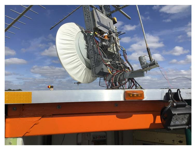
George uses a Cassegrain dish antenna for 10 GHz, which is a dish with an additional reflector that focuses the signal to the center of the parabolic reflector, right into the waveguide feed. The dish is two feet in diameter, and has a gain of about 28 dBd. A jeep spare wheel cover protects the dish when not in use.
